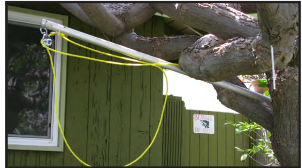
The lasso on a 10' light aluminum pole. Note pully at end of retrieving pole.
