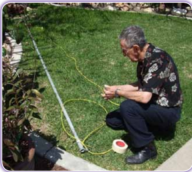
A very long pole with a rope, pulley, and a taped open loop (lasso).
