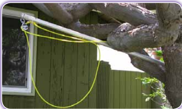
The lasso on a 10-foot, light aluminum pole. Note the pulley at the end of the retrieving pole.
