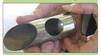
Put your thumb through the hole and firmly grasp the cutting as you make your slant cut.
